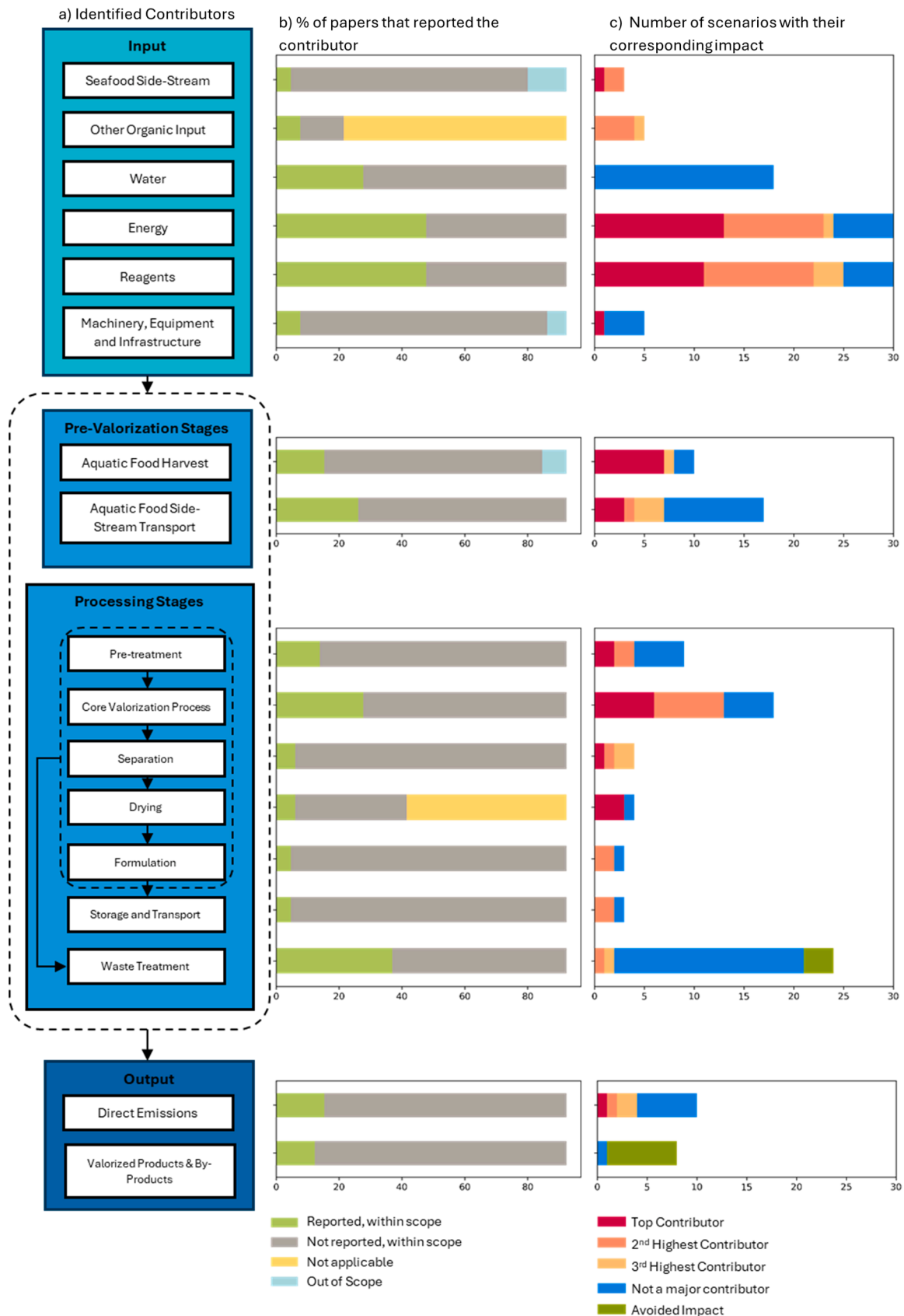
Fig. 6. Summary of contributors to Global Warming Potential (GWP) reported by papers in the results. (A) The bar graphs show the percentage of papers that reported the unit process, input, and output. It is also indicated where it will not be applicable. (B) The bar graphs show the impact of the unit process, inputs, and outputs reported by papers for each valorization scenario analyzed. Only valorization scenarios where included in the analysis (B); business as usual scenarios were not included.
