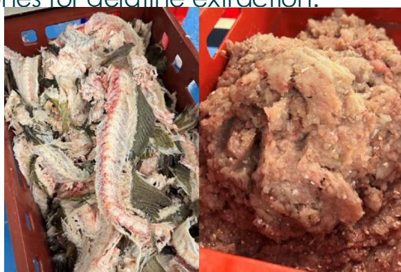
Cod backbones, bone fraction and soft tissue fraction after processing in the belt separator.
